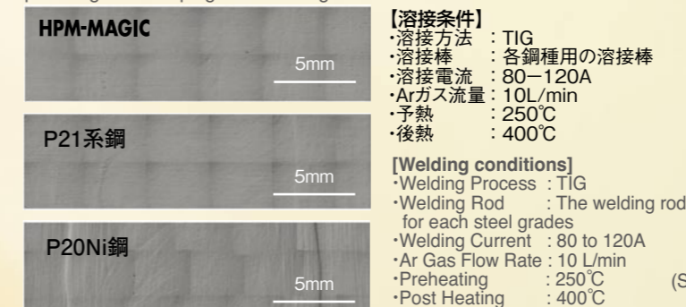
● 溶接後の磨き面の微分干渉像比較 Differential interference micrographs comparison of the polish surface after welding
